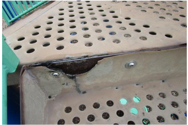
Wiggle Tube Slide - Cracked at top hood section - CLASS B HAZARD
