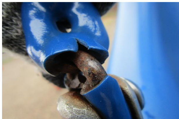
8ft. Swing Set (2Bay)(Landscape) - Chains worn at Inclusion seats - CLASS A HAZARD
