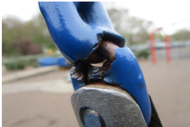
8ft. Swing Set (2Bay)(Landscape) - Chains worn at Inclusion seats - CLASS A HAZARD
