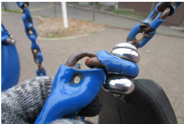
Freestanding Equipment 8ft. Swing Set (2Bays)(Landscape) - Chains worn at two belt seats - CLASS A HAZARD
