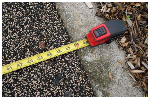
Sway Fun Glider - Use zone inadequate at 48" at rear - CLASS C HAZARD
