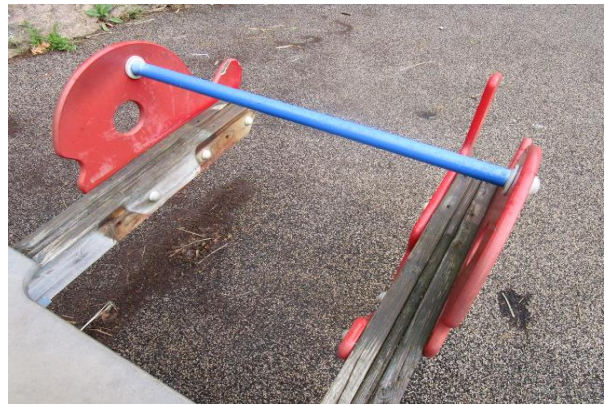
Multi-Spring see-Saw (Kompan) - One bolt cap cracked - MAINTENANCE
