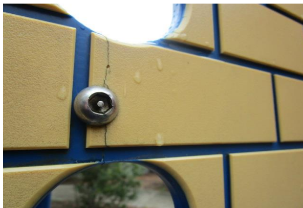
Curved Rung Ladder - Handhold panel cracked at bolts - MAINTENANCE
