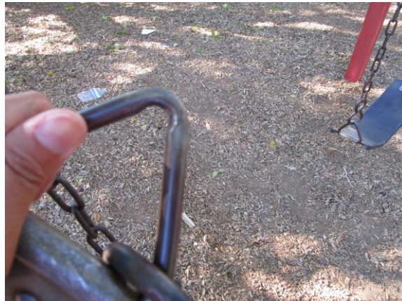
8ft. Swing Set - Eight clevises (below) & all chain starting to wear - MAINTENANCE
