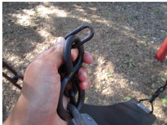
8ft. Swing Set - Eight clevises (below) & all chain starting to wear - MAINTENANCE
