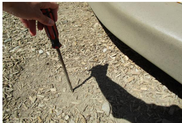
Surfacing - Insufficient at 0-2" - CLASS A HAZARD
