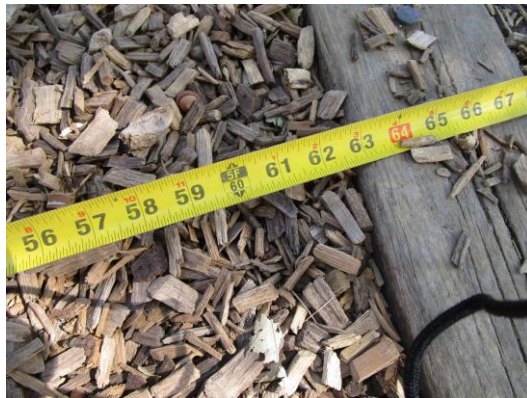
Use Zones - Inadequate, only 63" at Rumble Slide - CLASS C HAZARD
