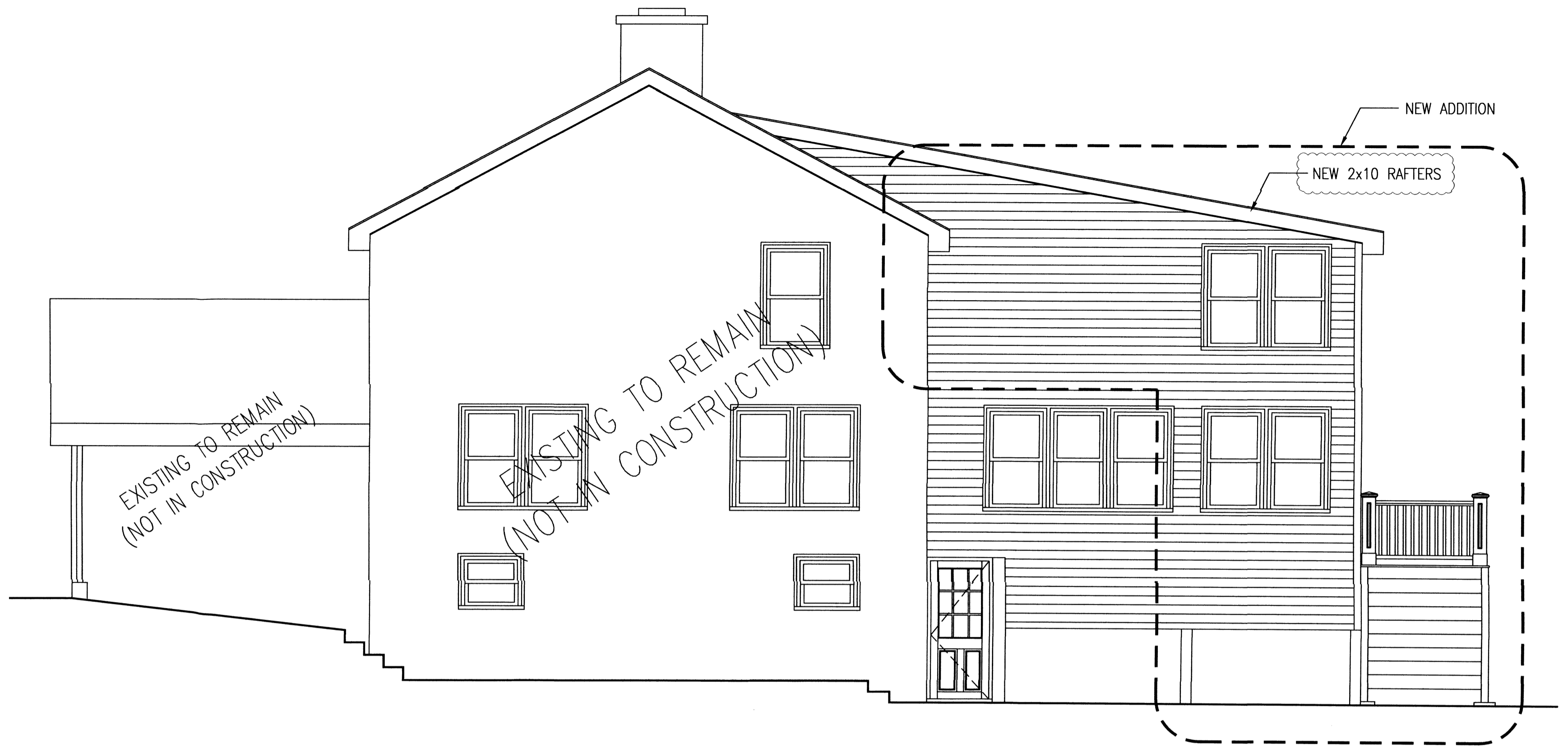
2B PROPOSED RIGHT ELEVATION A-4 1/4"=1'-0"
