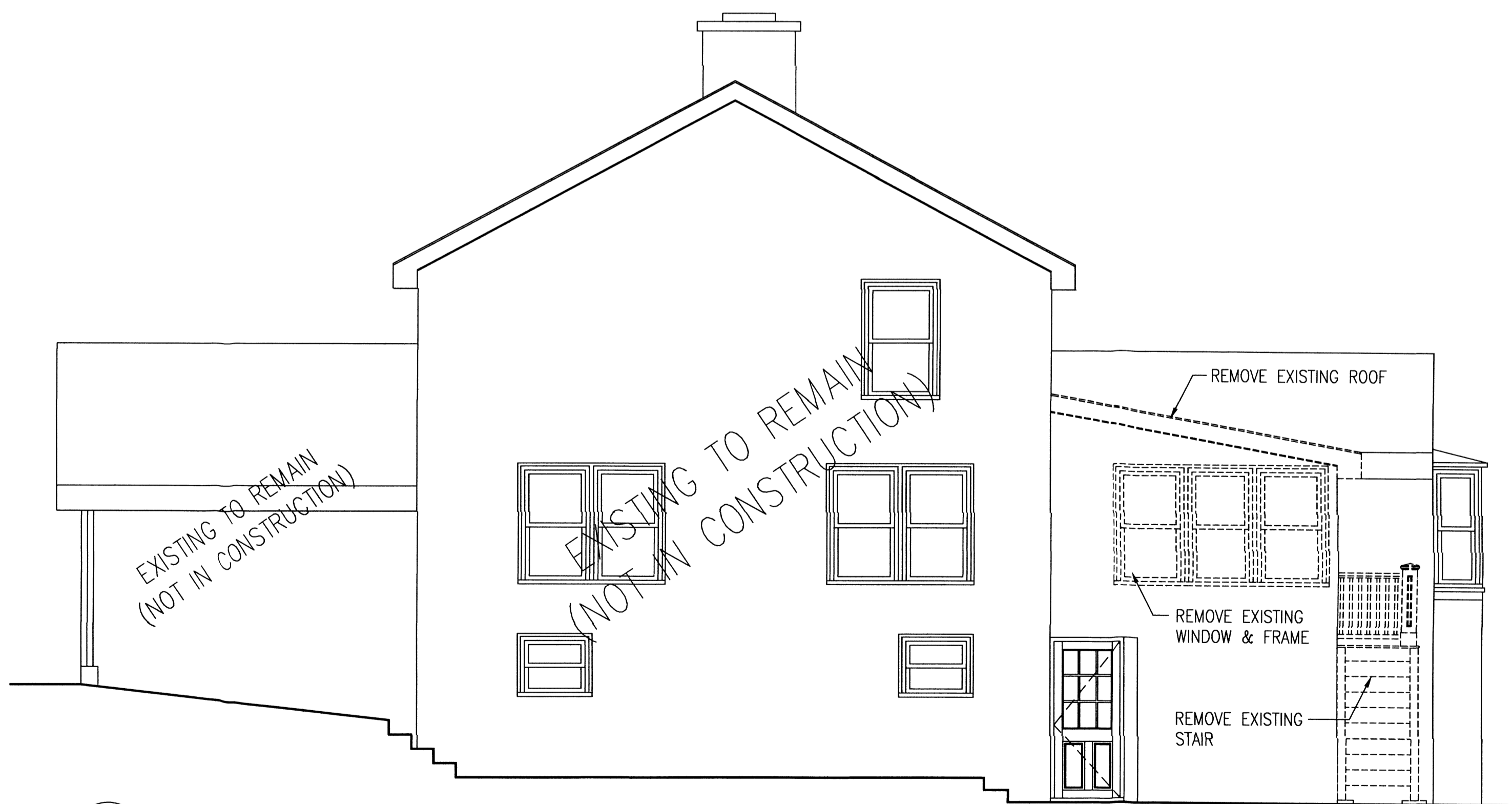
2A EXISTING RIGHT ELEVATION A-4 1/4"=1'-0"
