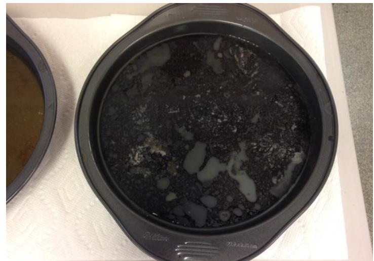
This Pan was NOT Dry Wiped with Paper Towels before Hot Water was put in the Pan.
