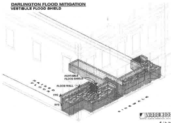
To provide additional protection against floodwater, removable watertight floodgates were incorporated into the buildings
