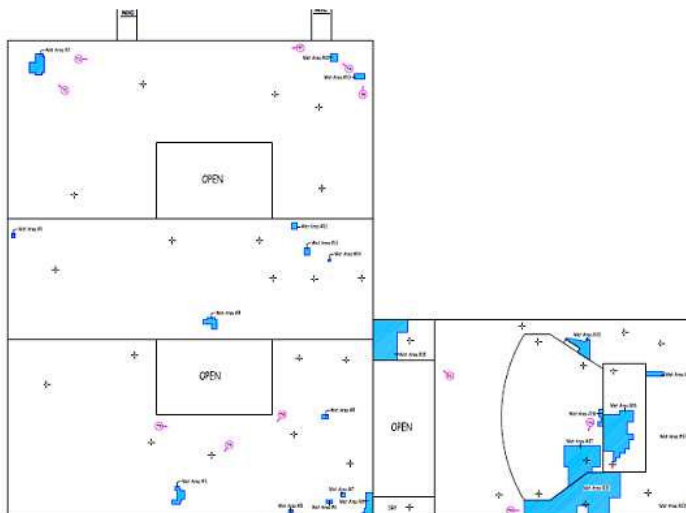
Roof moisture scan showing wet areas
