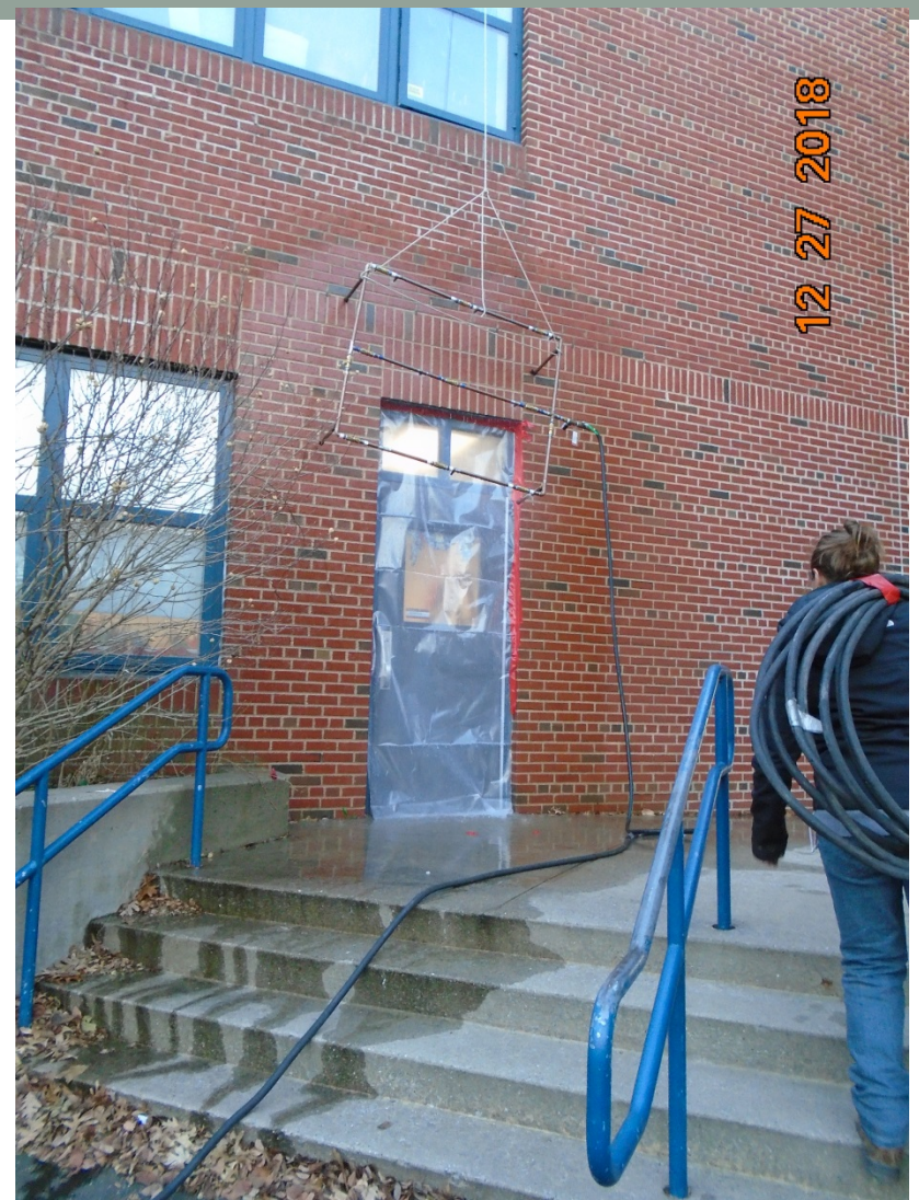
Engineers tested select windows and doors for water intrusion. December 27, 2018
